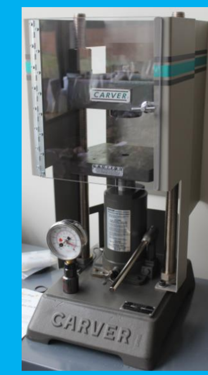
Carver 25 ton press for making pressed pellets for trace element analysis
