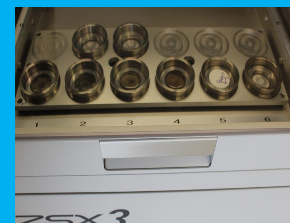
Glass fusion beads and pressed pellets in sample holders waiting analysis
