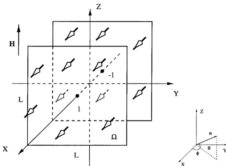
FIG. 1. Liquid crystal film confined between two plates with director field  $\mathbf{n}$  perpendicular to the plates. The magnetic field  $\mathbf{H}$  points in the  $z$ -direction.
