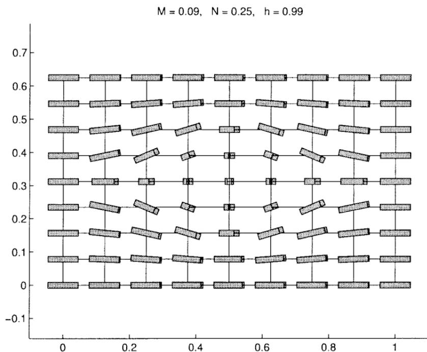
FIG. 2. A single period of the stripe phase as viewed from the direction of the magnetic field. The director field is periodic in the vertical direction and the glass plates bound the crystal from the right and from the left [6].
