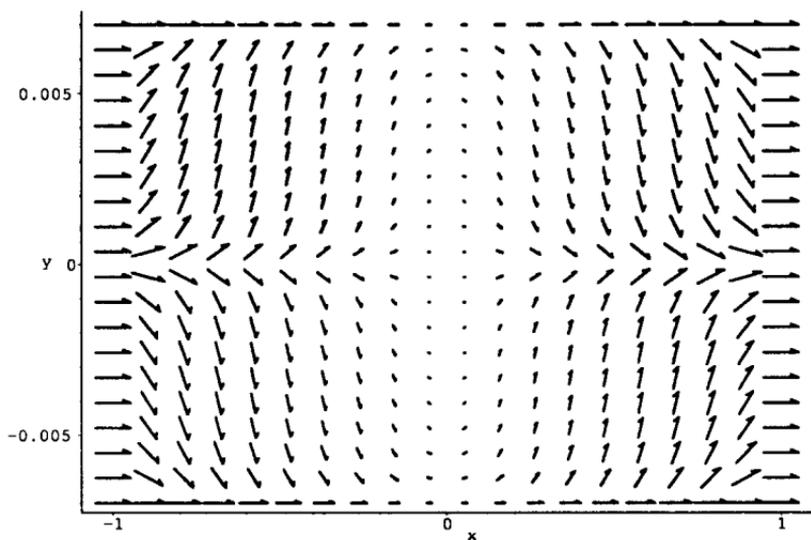
FIG. 4. A single period of a perturbation (20) of the Fréedericksz solution as viewed from the direction of the magnetic field.
