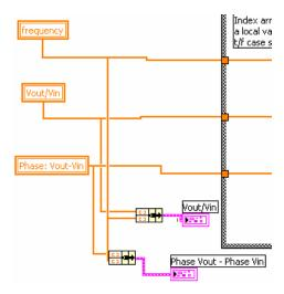
Next we have to take this data and make a ASCII text file = most generic form of file that can be read by just about anything. We will build a new array with all pieces of information (frequency, Vout/Vin, and phase difference) then transpose it (so EXCEL likes it – puts the arrays of data in columns instead of rows) and send this to the 'write file' part of our program.
