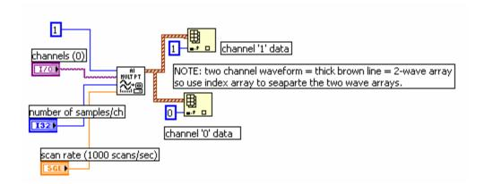
The outputs from the index arrays are just the individual waveforms from each channel.
