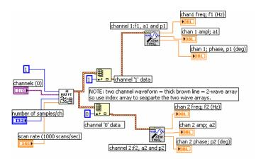
Now we can look at the actual data we are interested in,  $\frac{V_{out}}{V_{in}}$  and the relative phase (p1-p2) (the two frequencies should be the same... ie the driving or reference frequency).
