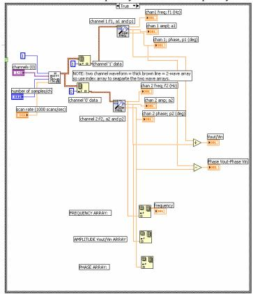
The way we get LabView to add the data for each new frequency is to make what amounts to a shift register for the case (true/false) we have. We used shifts registers to keep adding data from a 'for loop' earlier.
