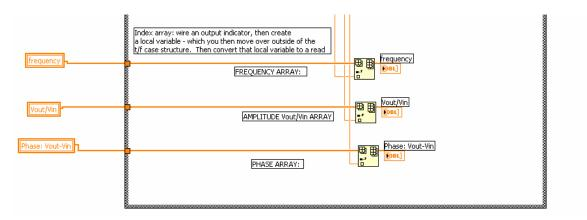
Now we will bundle together  $\frac{V_{out}}{V_{in}}$  vs frequency for one plot and (Phase Vout – Phase Vin) for a second plot.
