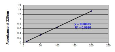
Figure 1. Calibration curve for the determination of copper in Anytown water.
