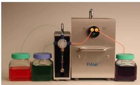
Flow injection analyzer (FIA): Image available at <http://www.flowinjection.com/whatsnew.html>
