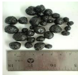
The Terra-Bond™ technology can be used to encapsulate hazardous, solid, finely divided waste materials within stable, discrete pellets
