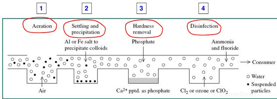
FIGURE 14-1 The common stages of purification of drinking water.
