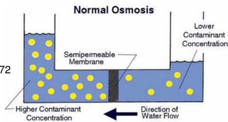
Water flows from a concentrated solution to a more dilute (usually just pure H<sub>2</sub>O) solution
