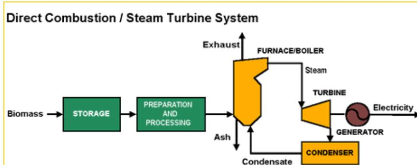
Diagram 1: In a direct combustion system, processed biomass is the boiler fuel that produces steam to operate a steam turbine and generator to make electricity.<sup>29</sup>
