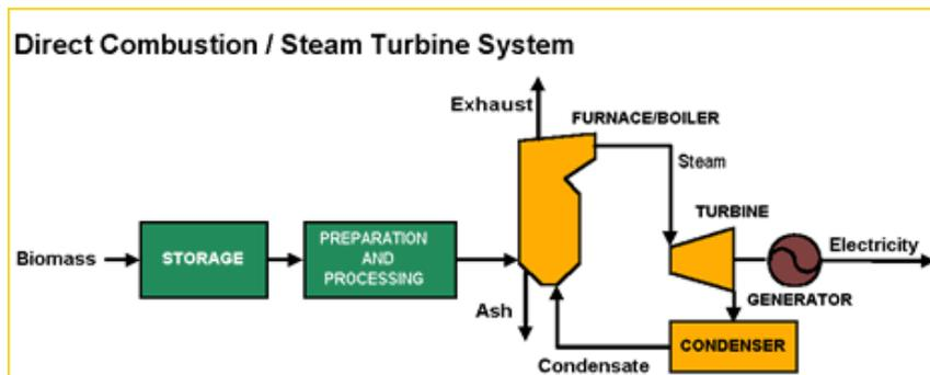
Diagram 1: In a direct combustion system, processed biomass is the boiler fuel that produces steam to operate a steam turbine and generator to make electricity.<sup>29</sup> Image available at [http://www.eere.energy.gov/de/biomass\\_power.html](http://www.eere.energy.gov/de/biomass_power.html)
